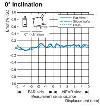
Note: The x-axis displacement indicates the measurement distance displayed by the amplifier unit. The measurement distance displayed by the amplifier unit takes the measurement center distance as 0, and the NEAR and FAR sides from the sensor are displayed by + and -, respectively.
