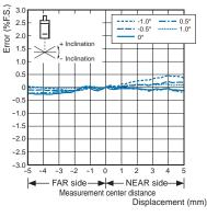
Side-to-side Inclination for Silicon Wafer
