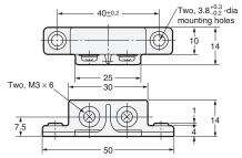
Note: Tighten each M3 screw of the terminal block to a torque of 0.59 N·m. max.
