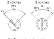
Note: The angles in parentheses are for automatic-reset models. FP: Free position
