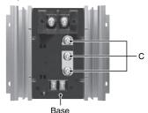
(4) Remove the connectors that connect the lead wires to the Thyristor Module, and remove the Module.
