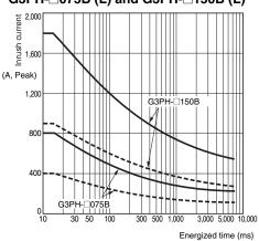
Keep the inrush current to below the inrush current resistance value (i.e., below the broken line) if it occurs repetitively.
